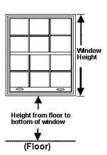
Measure window height and height from floor to bottom of window.
